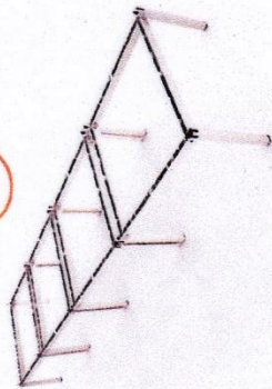
Lay out back row of frames
